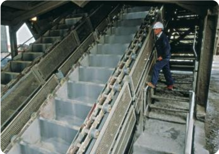
Special Double Strand Conveyor Chain is designed to give an enhanced chain life in the hot and dusty conditions of a Cement Clinker.
