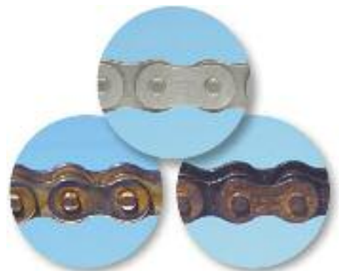
After 14 days in and out of a 5% saltwater solution (equivalent to sea water) it can be seen that the Hydro-Service® coating will extend the chain life compared to conventional nickel plating or carbon steel in more challenging applications.
